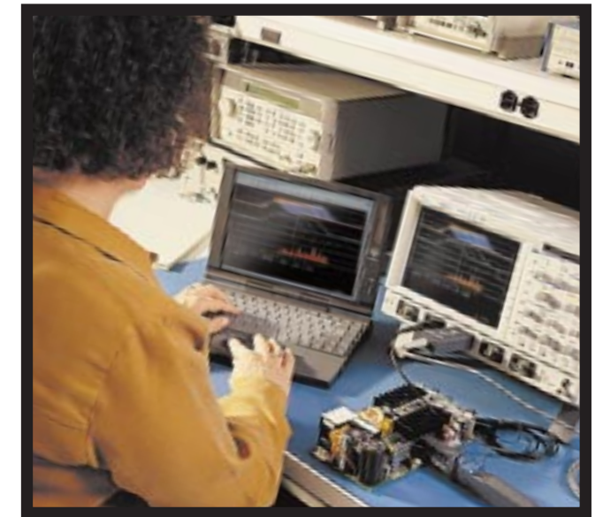
All it takes is a PC with Windows 95, 98, or NT and a GPIB, RS-232-C, or New 10 Base-T Ethernet option.
